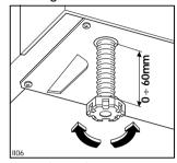
The recess height may be anywhere between 820 and 880 mm from the floor since the dishwasher incorporates levelling feet adjustable over a wide range (max 60 mm).
